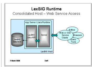
The LexBIG API is designed with web and grid-level enablement in mind. This diagram depicts deployments that wrap the current API to allow the runtime to be accessed through web or grid services.
