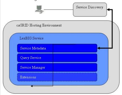
The LexBIG architecture provides the underpinnings LexBIG services to be made accessible through the caGRID environment in the future, where LexBIG services might optionally be deployed in a caGRID Globus container. caGrid provides a Globus service for service registration and discovery. LexBIG services deployed to the grid would be registered in the NCICB registry and be searchable through the NCICB index service.
