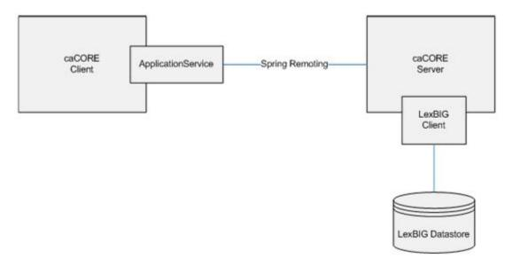
The DLB environment will be configured on the caCORE LexEVS Server (http://lexevsapi.nci.nic.gov/lexevsapi50). This will give the server access to the LexBIG database and other resources. The client must therefore go through the caCORE LexEVS server to access any LexBIG data.
