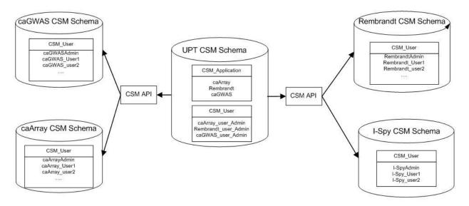
The UPT Schema has database connection and administrator information for each application database. The CSM applications are included (caArray, Rembrandt, and caGWAS in the example), and the CSM\_User admins. For each application, the schema lists the CSM admin and users.
