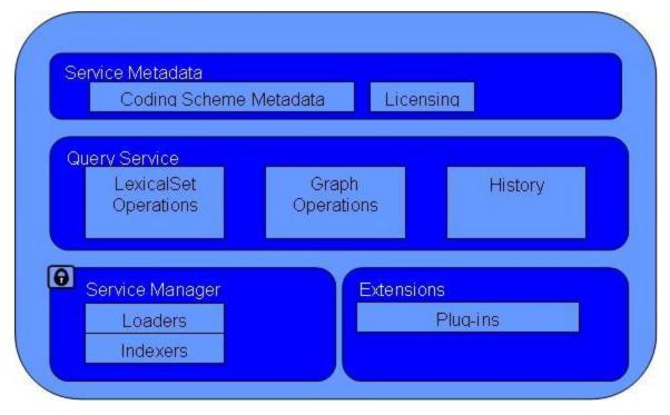
The LexBIG Service is designed to run standalone or as part of a larger network of services. It is comprised of four primary subsystems: Service Management, Service Metadata, Query Operations, and Extensions.
