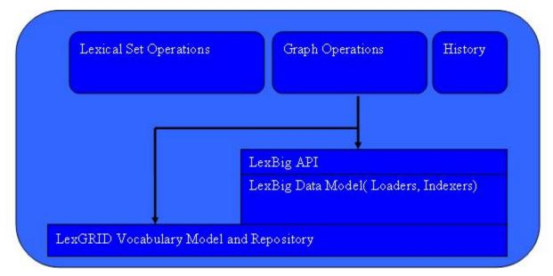
This subsystem provides the functionality required to fulfill caCORE/EVS and other vocabulary requests. The Query Service is comprised of Lexical Operations, Graph Operations, Metadata, and History Operations.
